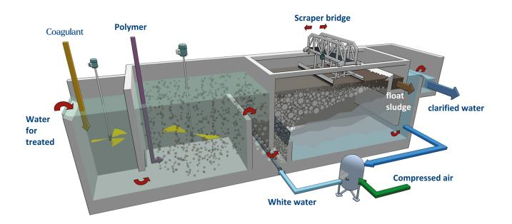
AEROFLUX® technology is a process based on the principle of Dissolved Air Flotation (DAF) used for the clarification of drinking water following coagulation-flocculation.
