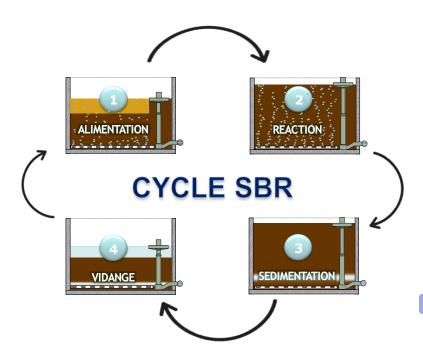
By integrating the clarification process into the biological treatment cells, **CYCLAFLUX**<sup>®</sup>:
