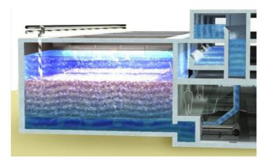
The principle of upflow co-current biofiltration of water and air on a material denser than water and non-compressible, combined with the intrinsic characteristics of biozzolane®, allows for high-speed operation without material compaction and with excellent performance.
