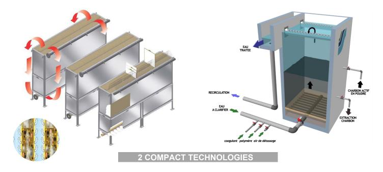
Membrane bioreactors offer higher pollutant and micropollutant removal efficiencies compared to conventional installations. This improved performance is not only due to the quality of effluent filtration but also achieved on the dissolved portion of the effluent. This enhanced performance, compared to tertiary filtration, is a result of various phenomena related to:
